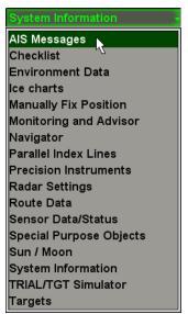
In the list, which will open up, select AIS Messages line and press the left trackball button.
