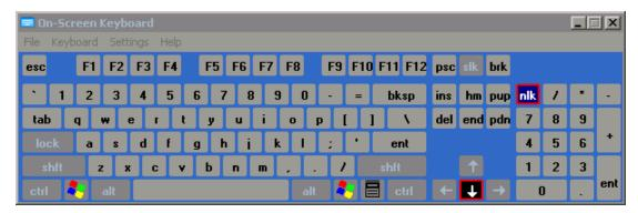
The virtual keyboard is shown in the bottom part of the Control panel and can be moved within it. To do this, position the free cursor on the virtual keyboard as shown below, and press the left trackball button. Holding the left trackball button, move the virtual keyboard to the necessary place so that it does not obscure the necessary input box.
