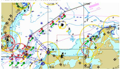
The reference point will be shown on the Chart Panel in the form of two blue circles. The blue dashed line connects the WPT WOL and its corresponding reference point.
