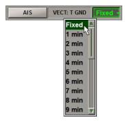
Select the required vector length (see document *Multi-Functional Display (v. 3.00.340). Functional Description, Chapter 3*, section *Own Ship Motion Data*, paragraph *Own Ship Motion Vectors*) from the list, which will open up and press the left trackball button.
