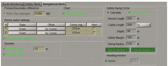
Check the checkboxes in the Alert column to turn on the alert generation as the ship sails beyond the set distances.
