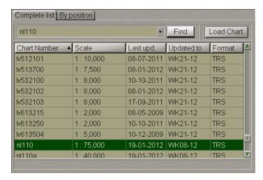
The necessary chart will be highlighted in the table. Press Load Chart button, the selected chart will be loaded in the Chart panel.
