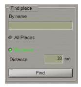
Press Find button. Position the graphic cursor, which will appear, on the point within the Chart panel which will be the centre of the area coverage circle.
