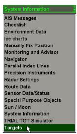
In the list, which will open up, select Targets line and press the left trackball button.
