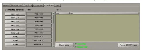
This page is intended for displaying and recording of the IEC 61162-1, 61993-2, and proprietary formats and similar text messages/sentences provided to the MFD from the external sensors and displaying of the sentences transmitted by the MFD to the external devices.
