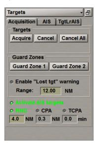
Check the Activate AIS targets checkbox for the automatic activation of sleeping AIS targets by one of the following criteria:
