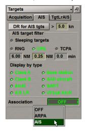
Select from the Assotiation drop-down list the targets which will be displayed after the association on the ECDIS task screen (e.g. AIS).
