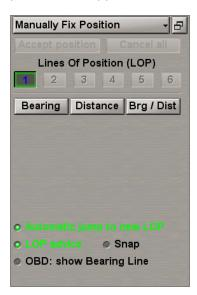
The OBD continuously transmits bearing information to the MFD. This allows the ECDIS task screen to provide a real-time display of an Optical Bearing Line – showing what the OBD operator is looking/pointing at. Press OBD: show Bearing Line button.
