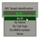
In the list, which will open up, select the necessary identifier or None to declutter the Chart panel. Press the left trackball button. Targets will be displayed on the Chart panel with the selected identifier, and its name will be shown on the button.
