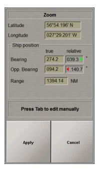
The first press on the Apply button set the top left corner of the zoom area in the cursor position, the second press turns on the zoom mode.
