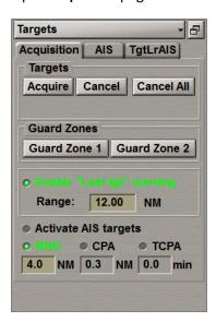
Use the Range input box to set the distance within which the Lost Tgt warning will be generated when the ARPA or AIS loses a target. Beyond the set distance the lost targets are not at all displayed on the ECDIS task screen any more without warning.
