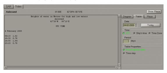
In Date line of **Table** tab, select the date starting from which the tidal heights will be calculated. Use **Period** input line to enter the period which tidal heights are required to be calculated for.
