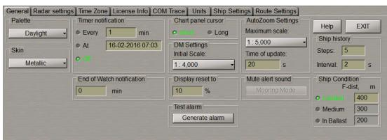
Use the tab in the top part of Config panel, which will open up, to switch to General page.
