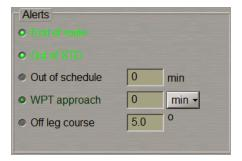
Alerts group is intended for turning on/off and setting of safety parameters for the alert generation during the sailing along the route and according to the schedule:
