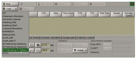
In the list, which will open up, select the route required to be loaded in edition mode, and press the left trackball\mouse button.
