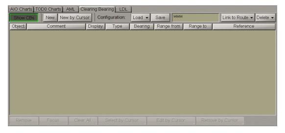
Press the Show CBs button to display Clearing Bearings (CBs) on the ECDIS task screen.
