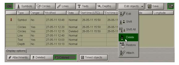
Position the acquisition marker, which will appear, on the object to be deleted (the first character of a text object or a point in a line or area type object).
