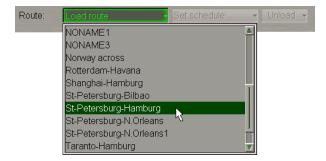
Select the required route and press left trackball button. The selected route will be loaded for sailing in the Chart panel, and its name will be displayed on the button. The route loaded for sailing will be shown in red colour.
