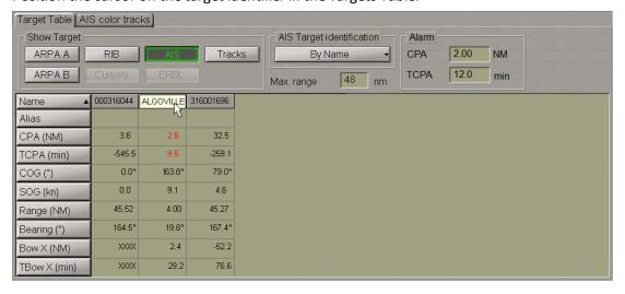
The hint will display the name of the AIS object if it is contained in the messages transmitted by the AIS object.
