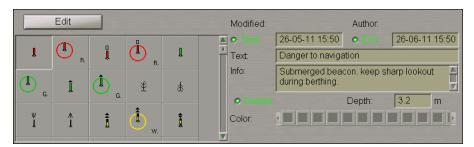
Edit the updating object parameters so as display time ("Temporary updating" attribute), text ("Text" attribute), required information ("Object information" attribute), "Danger to navigation" attribute and required depth value ("Object depth" attribute) (see paragraph *Plotting Point Type Object*).
