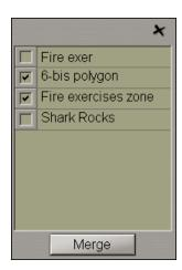
In the window which will open up, check the checkboxes next to the maps which should be merged. Press the Merge button.
