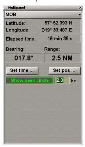
The Show seek circle button is enabled by default. Use the input box to the right of the button to enter the seek circle expansion rate different from 0.
