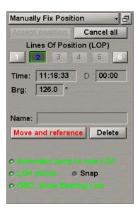
Data from the OBD will be displayed in the Brg input boxes and can be subsequently used for further calculations (see above).
