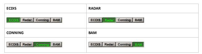
3. From the Transas Integrator. To turn on the ECDIS task from the Transas Integrator utility, press ECDIS button
