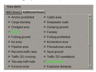
Select the required areas by checking the appropriate checkboxes in IMO Areas tab.
