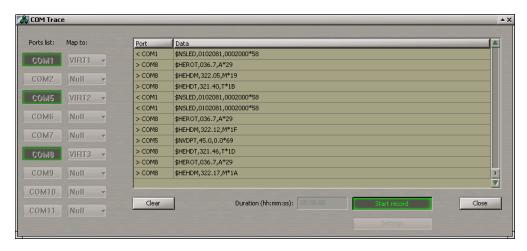
The comtrace.\_\_\_\_\_ file recording will be made from all the turned on COM ports during the time specified in the Duration window (30 minutes by default). If it is necessary to interrupt the recording, press the Start record button again. After the end of the recording, the Start record button will be automatically disabled.
