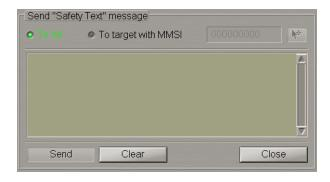
Set the identifier of the addressee of the message to be sent. To transmit a message to all the ships in the radio coverage area, check **To All** checkbox.
