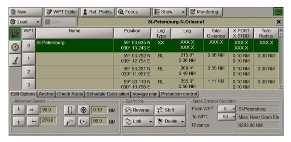
Several routes can be loaded simultaneously in the editing mode. As a button with route name is pressed, the route becomes active and can be edited on the screen by using the graphic editor.
