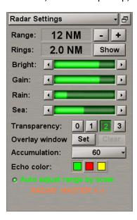
In **Radar Settings** display which will open up, set the range scale. To do this, use the buttons to the right of **Range** input window.
