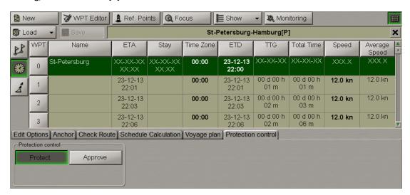
The protected route can neither be saved under the previous name, nor deleted. If saved under an altered name, the route loses its "Protected" status.
