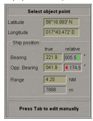
Position the acquisition marker in the reference point of the Clearing Bearing and press the left trackball button, the acquisition marker will change its form to the graphic cursor.
