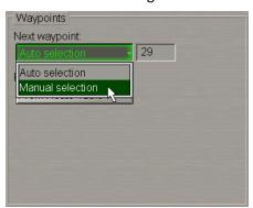
In the list, which will open up, select Manual selection and press the left trackball button. Use the activated input line to enter the next WPT number.
