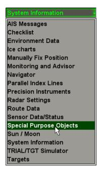
In the list, which will open up, select Special Purpose Objects line and press the left trackball button.
