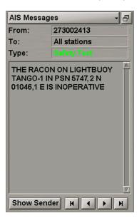
In AIS Messages display, which will open up, read the received message. Use buttons to view the received messages.
