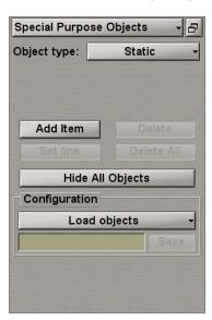
This MFD functionality enables special purpose objects (SPO), mobile and fixed, with certain features to be created and referenced to an electronic chart with the purpose of their further monitoring and obtaining of auxiliary information.
