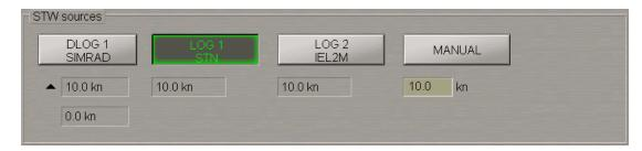
**STW** sources group is designed for selection a source of speed through the water. The group shows all the connected speed through the water sensors.
